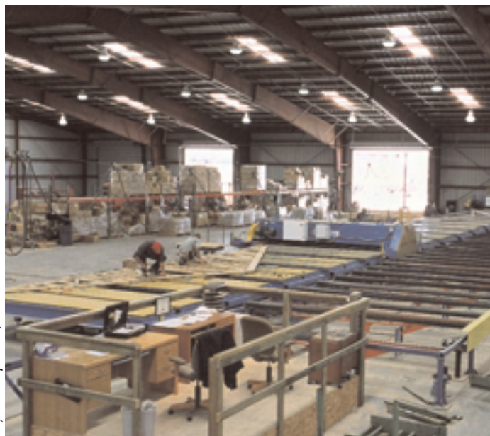
The Hayward plant features infrared-sensor lighting systems that automatically adjust the lighting to daylight conditions. A series of skylights mounted between the PV modules on the east-facing roof provide the daylight.
