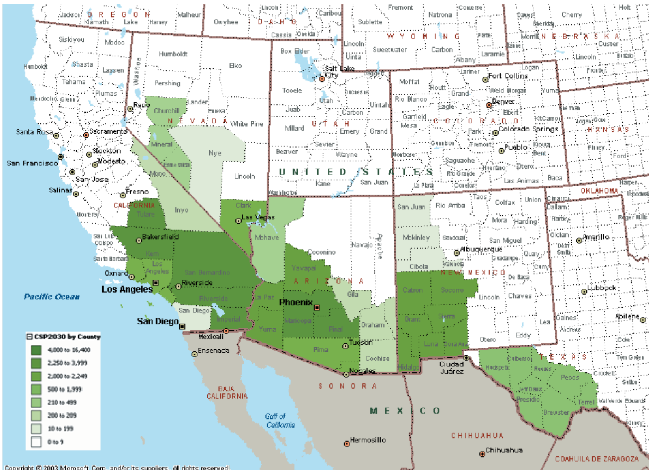
Figure 9. Market deployment of 80 GW of CSP assuming a 30% investment tax credit and a carbon value of $35 per ton of CO 2 .
